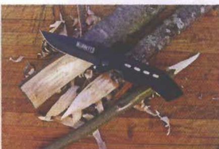
The M50 proved to have excellent edge geometry for basic cutting chores like working with both green and seasoned hardwood. Resharpening was a cinch with a Norton benchstone.
